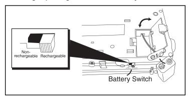
The Emergency Alert Radio can use either a 9 volt alkaline or a Nickel Cadmium (Ni-Cd) rechargeable battery as its backup power source.
